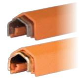
Continuous roll formed inverted "V" cross section encased by an insulating PVC cover. Splice kit included with the price of conductor. Operating Temperature:  $-10^{\circ}$  F to  $160^{\circ}$  F. Bars are 15.0 ft (4.57 m) long
