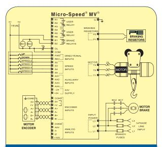
UP and DOWN limit switches can be placed in various locations depending on application requirements. Lights or alarms can be driven by user relays 1 or 2. Two optically isolated Motors & Encoders are also available from
