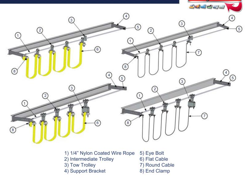
Wire rope festoon systems are ideal for light duty applications with limited distance and speed requirements where C-track cannot be installed. Choose from a complete range of trolleys based on your project demands. Systems can be purchased as complete packages or as individual components. Complete systems include the wire rope, trolleys, end clamp, rope clamps, thimbles and eye bolts.
