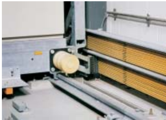
Conductor rail system in a high bay storage
