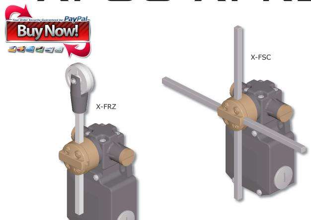
Position limit switches are designed to control the movement of overhead travelling cranes, hoists and machine tools. They operate as auxiliary controllers of electrical motors through power interfaces, such as contactors or PLCs.
